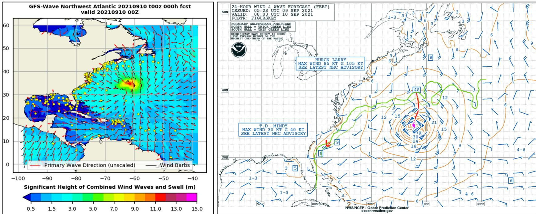
Figure 8. GFS-Wave significant wave height model analysis (m, left) and NOAA Ocean Prediction Center wind and wave 24-h forecast (ft, right) valid at 0000 UTC 10 September. Note the large wave and swell field (red arrows in left image) extending from Hurricane Larry that covers most of the western Atlantic. The swells were responsible for high surf and rip currents along many of the western Atlantic beaches and resulted in 5 direct drowning fatalities.
