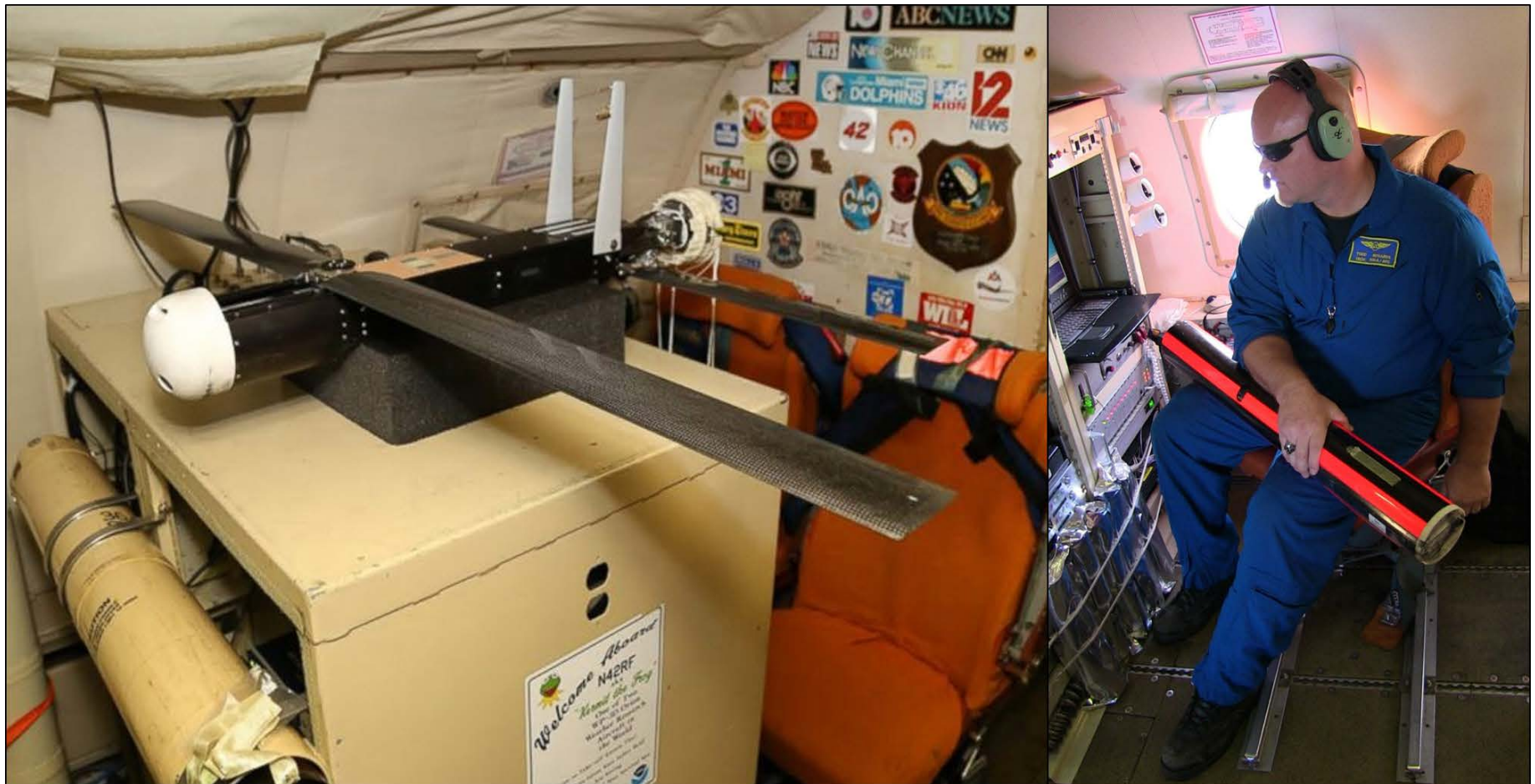
Figure 9. Coyote UAV, a component of the Small Unmanned Aircraft Vehicle Experiment (SUAVE), is displayed in flight mode (left) and is ready to be released by NOAA WP-3D Hurricane Hunter flight crewman (right) into the eye of Hurricane Edouard on 16 September. Pictures courtesy NOAA-AOML Hurricane Research Division.
