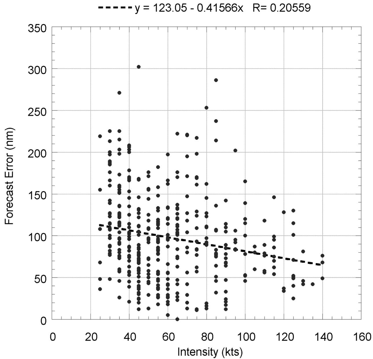
Fig. 63. GUNA 48-h track forecast error vs. initial TC intensity for 2001-2003 eastern North Pacific
