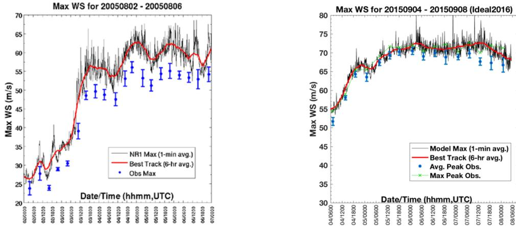
Figure 1: Undersampling results for HNR1 (left) and the new idealized simulation of an intense hurricane (right). Black curve shows peak 1-min mean wind every 6 or 5 min, respectively. Red curve shows running 6-hour mean. Dates for the idealized storm are fictional but used for comparison.
