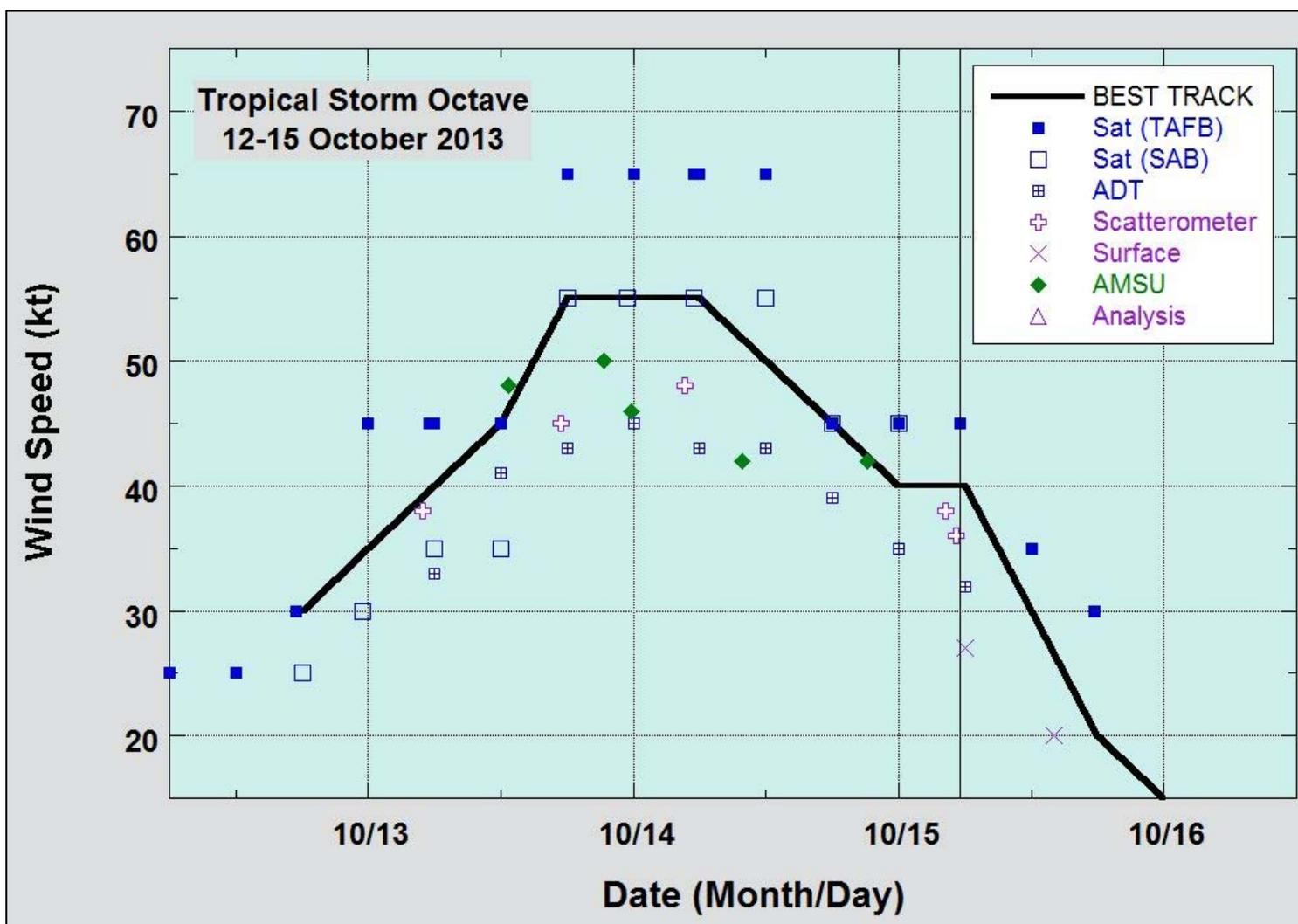
Figure 2. Selected wind observations and best track maximum sustained surface wind speed curve for Tropical Storm Octave, 12-15 October 2013. Advanced Dvorak Technique estimates represent the Current Intensity at the nominal observation time. AMSU intensity estimates are from the Cooperative Institute for Meteorological Satellite Studies technique. Dashed vertical lines correspond to 0000 UTC, and the solid vertical line corresponds to landfall.
