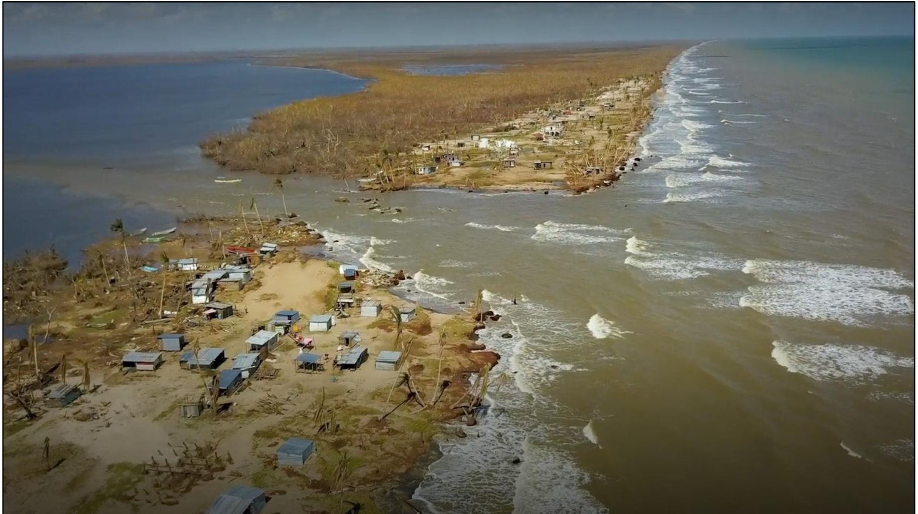
Figure 19. Cutout of barrier island caused by Hurricane Iota's storm surge at Haulover, Nicaragua. (viewing north -- picture courtesy *New York Times*)
