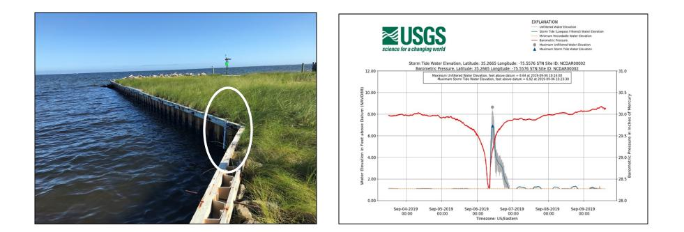
Figure 8. (a) A USGS pressure sensor installed on a bulkhead on Pamlico Sound in Buxton, NC (highlighted by the white ellipse). (b) Instantaneous water level (gray, ft above NAVD88), wave-filtered water level (blue, ft above NAVD88) and barometric pressure (red, in Hg) recorded from the sensor. Images courtesy of the USGS.
