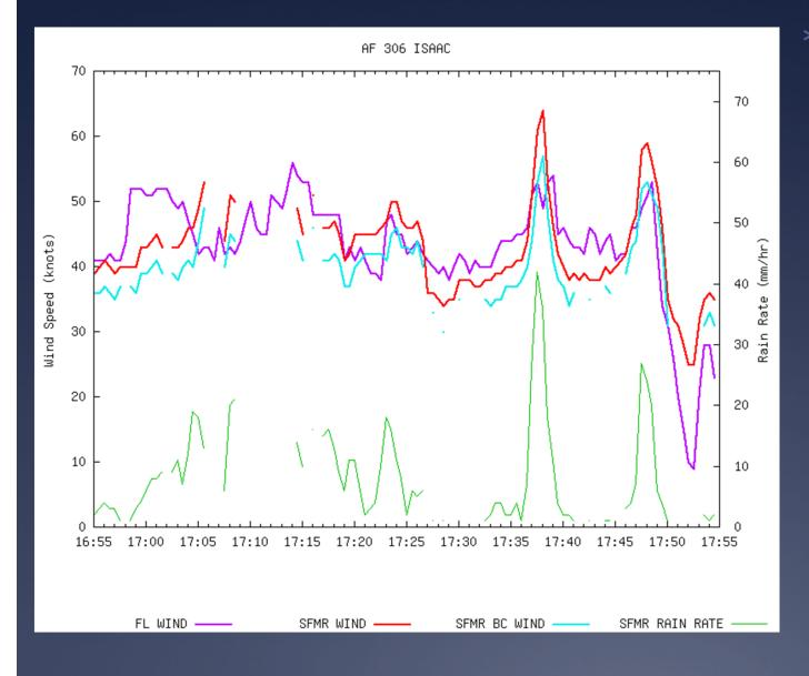
Rain spike at 1738Z causes raw SFMR wind of 64 kt, while biascorrected value is 58 <u>kt.</u>
