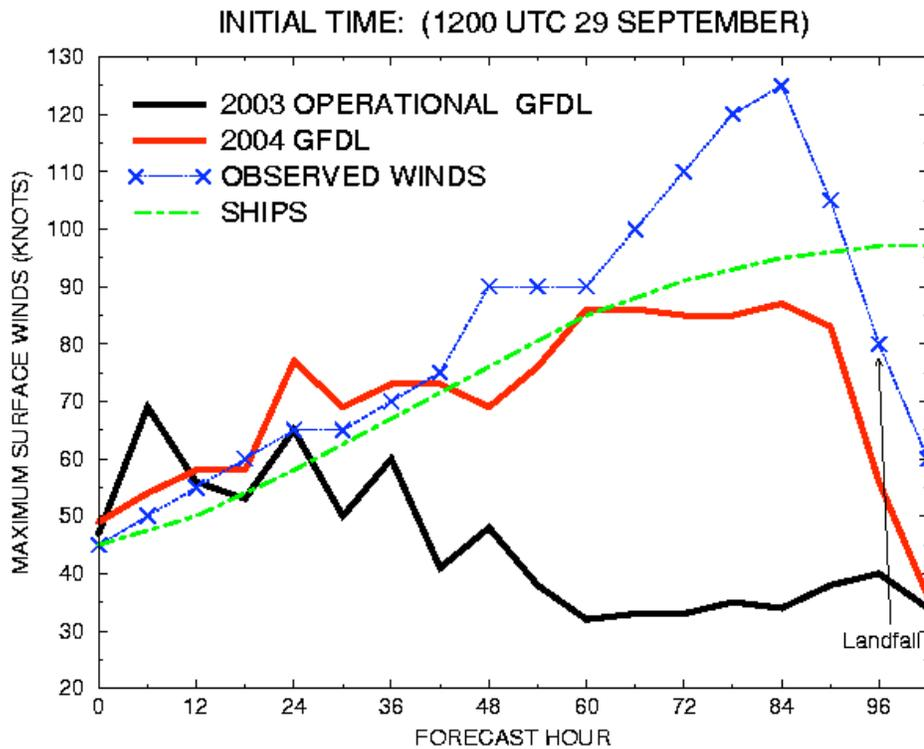
Figure 2 Predicted maximum surface winds (knots) for Hurricane Lili (Initial time: 1200 UTC 29 September, 2002) for the current operational GFDL model (black line), the new 2004 model (red line) compared to the observed winds (blue dashed line, X) and the SHIPS model (green dashed-dotted line).
