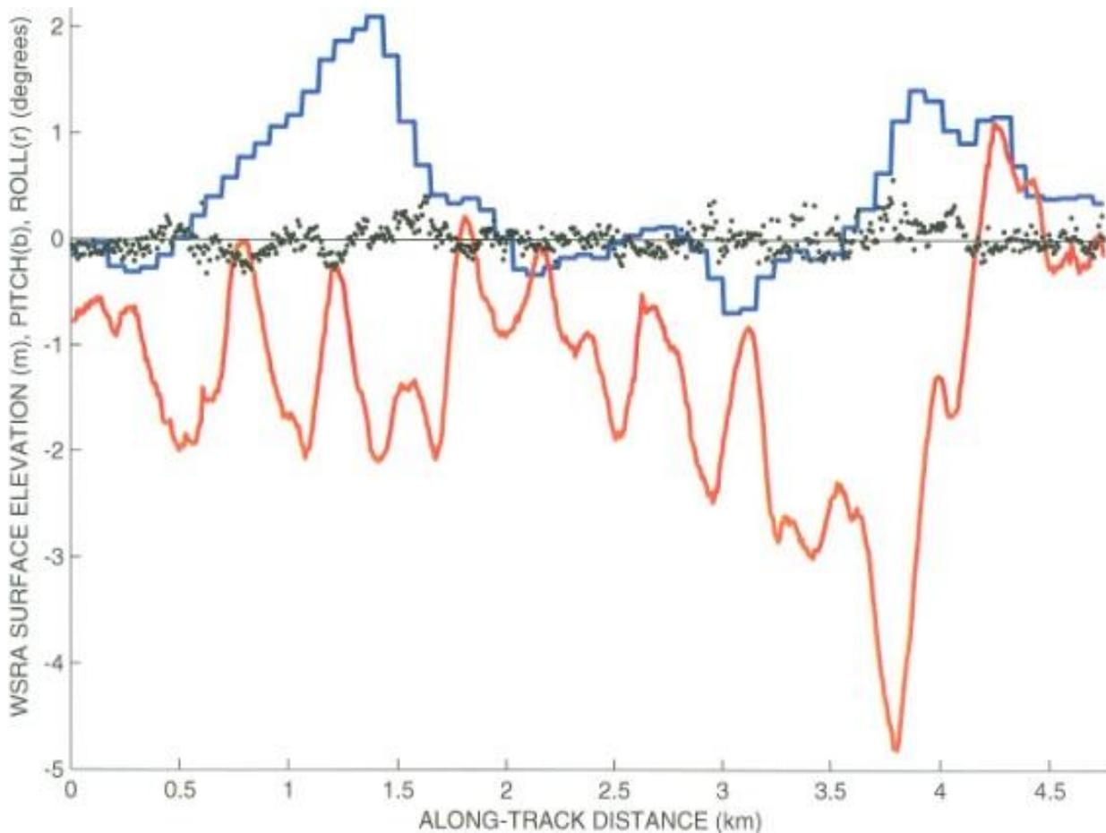
**Figure 4. Curves show the aircraft pitch (blue) and roll (red) variation for the highlighted flight segment over Tampa Bay and dots represent the residual error  $E_{RES}$  as defined in equation (2).**
