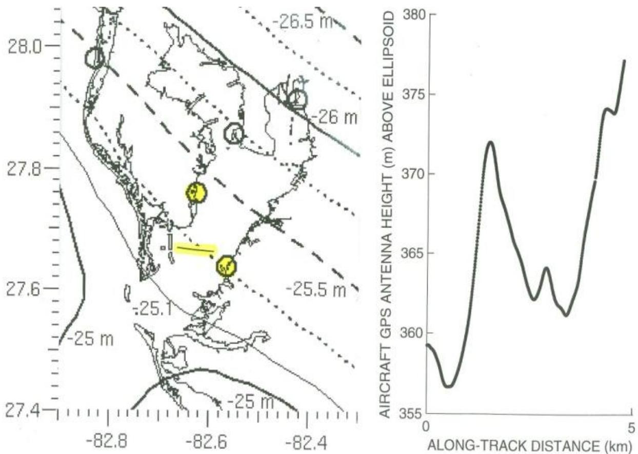
**Figure 3. Left panel shows contours of geoid height relative to the ellipsoid in the Tampa Bay area. Right panel shows the GPS measured aircraft height above the ellipsoid along the straight 5-km flight segment yellow-highlighted in the left panel.**
