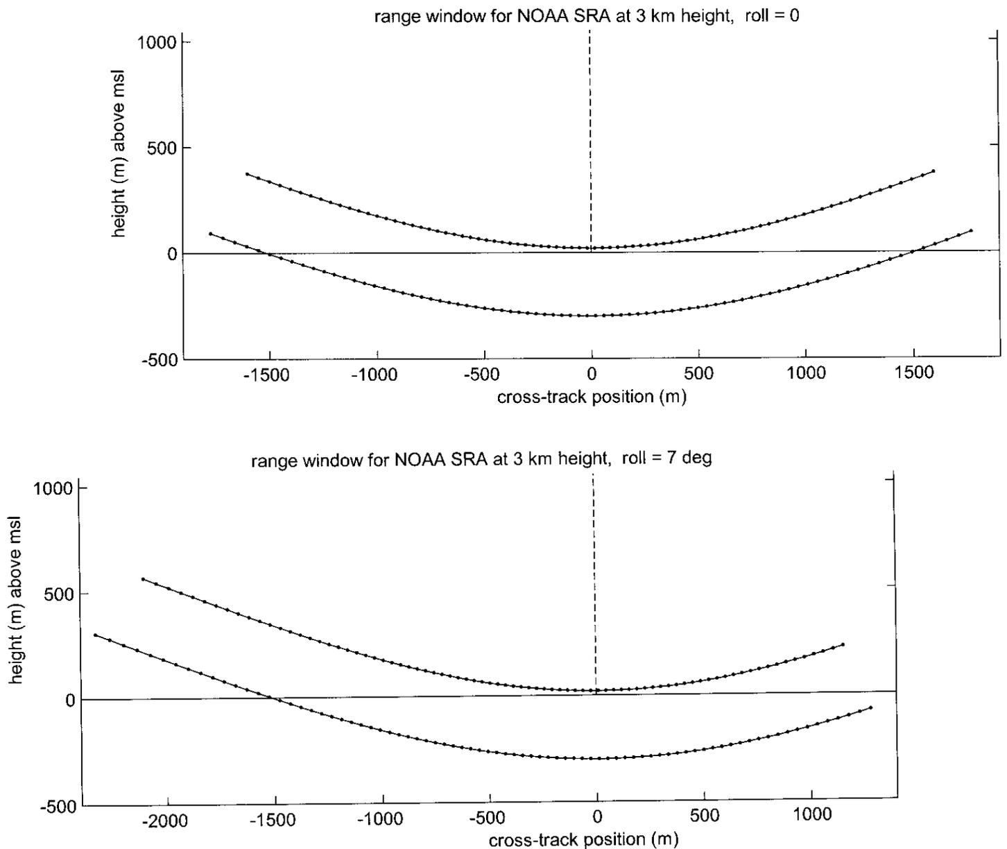
Figure 3. Range window position relative to msl for aircraft roll attitudes of  $0^\circ$  and  $7^\circ$ .
