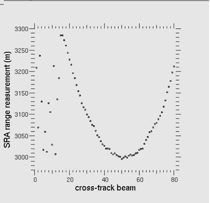
Figure 2. Simulated centroid range measurements.
