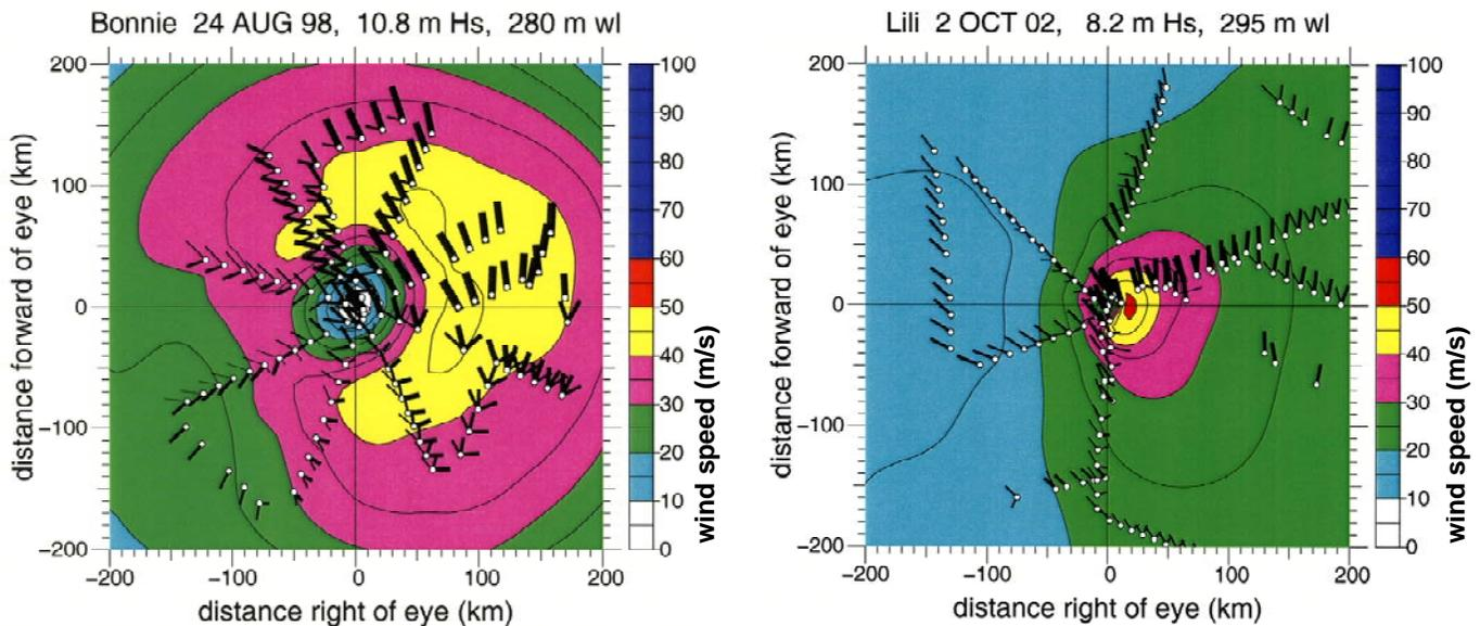
Black radials extend in the wave propagation direction a distance proportional to the ocean wavelength ( $wl$ ). Their width is proportional to the significant wave height ( $H_s$ ). Wind contours at 5 m/s, color changes at 10 m/s intervals.
