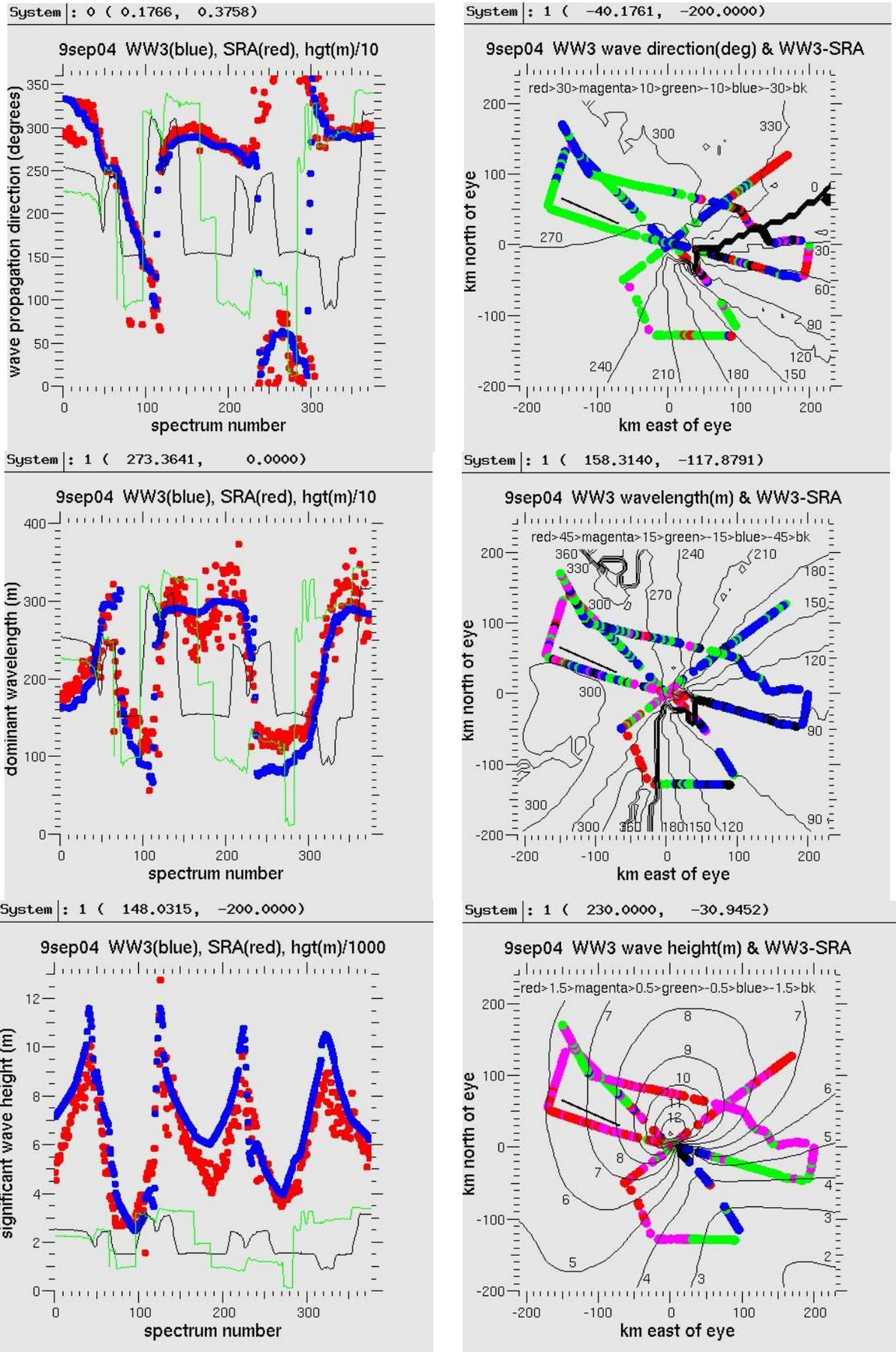
Figure 6. SRA wave field parameter comparison with WaveWatch III model output for Hurricane Ivan.
