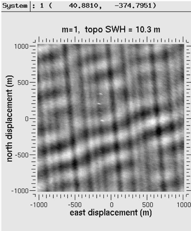
Figure 4. SRA measured wave topography.
