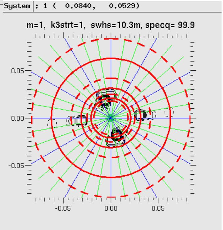
Figure 5. Directional wave spectrum from the SRA wave topography shown in Figure 4.
