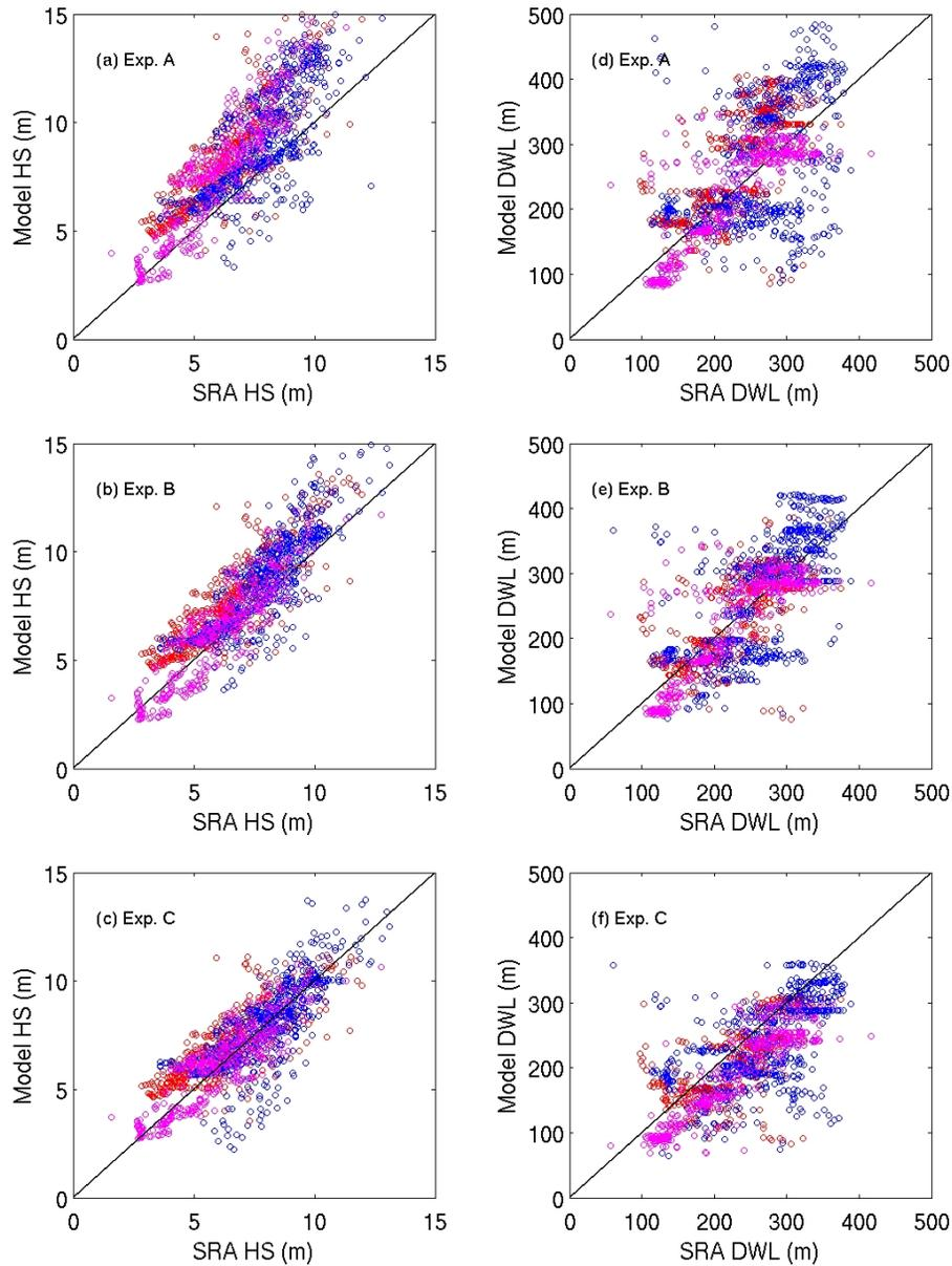
**Figure 2.** Model significant wave height ( $H_s$ ) vs. SRA measurements (left panels); and model dominant wave length (DWL) vs. SRA measurements (right panels) for (d) Exp. A with original WW3 drag coefficient, (e) Exp. B with new drag coefficient based on the coupled wind wave model, and (f) Exp. C with the new drag coefficient and with the effect of ocean currents. The magenta, red, and blue circles correspond to the calculation period of September 9, 12 and 14-15.
