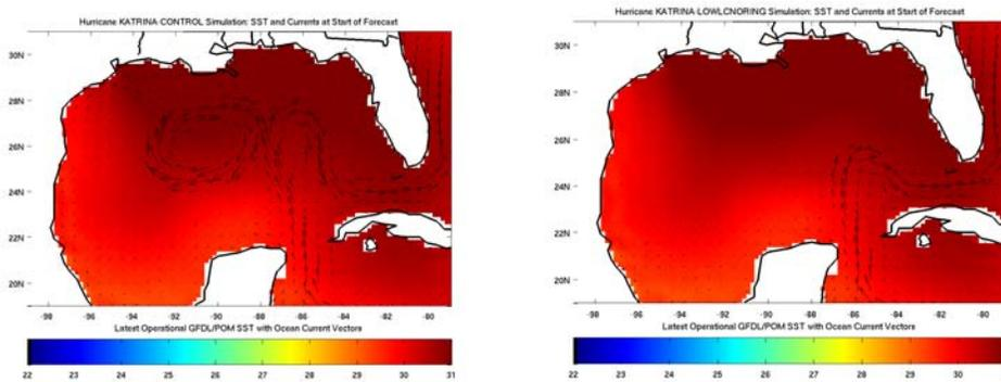
**Figure 3.** SST and surface currents for Hurricane Katrina coupled GFDL model forecasts with the Loop Current and a warm core ring initialized based on altimetry to represent the actual location as of 26 August 2005 (left panel) and a modified Hurricane Katrina coupled GFDL model forecast in which the Loop Current is initialized in its climatological position, and no warm core ring is assimilated (right panel).
