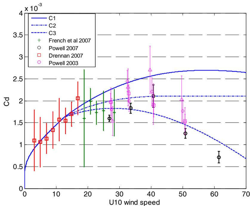
**Figure 1.** Three sea state independent drag coefficient formulae (C1: parameterization implemented into the operational HWRF and GFDL model; C2: proposed drag formula to saturate at high winds, C3: proposed drag formula to decrease at high wind) are compared with previous observations (symbols with error bars). Different symbols of Powell (2003) indicate estimates from different wind profile ranges.
