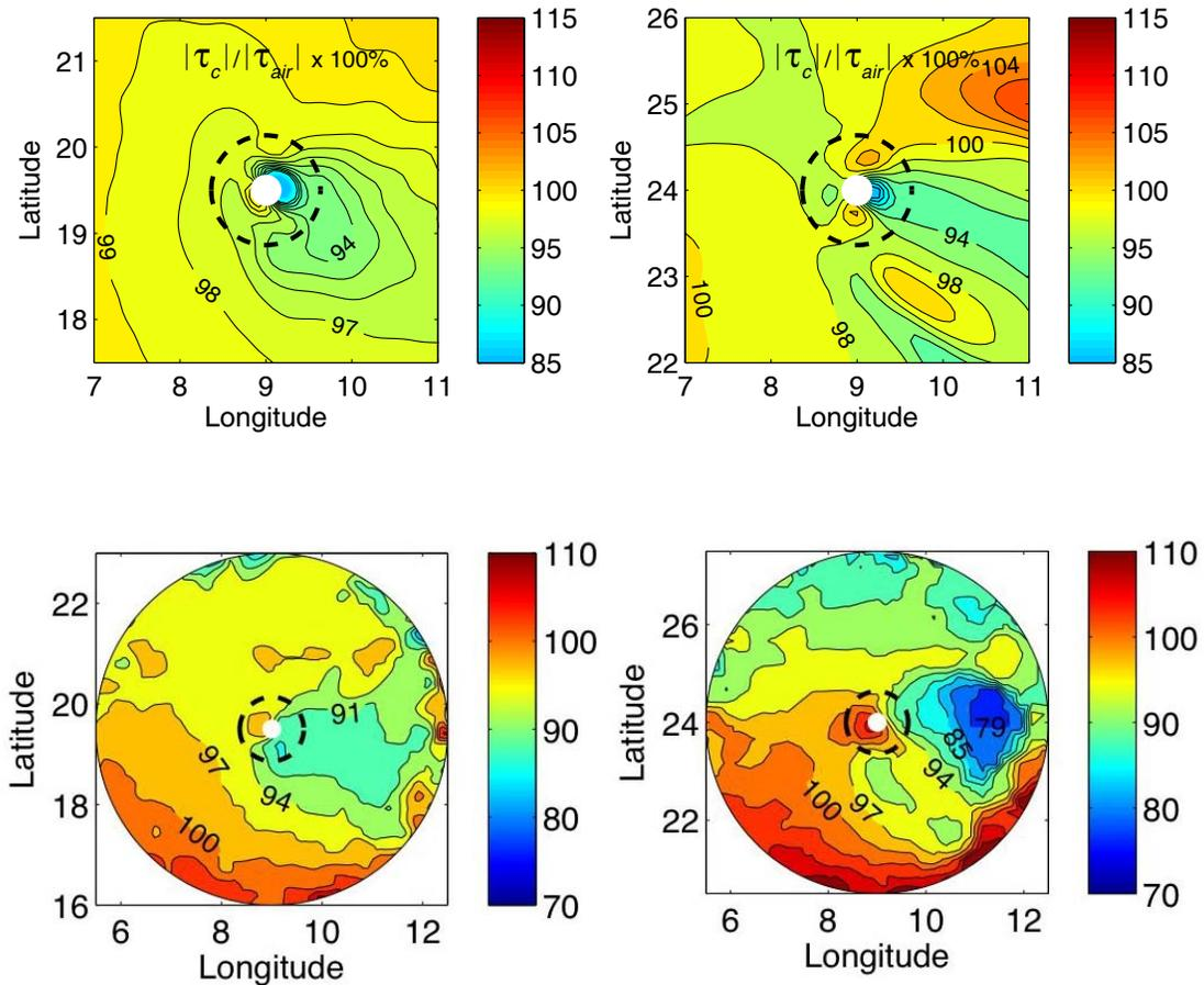
**Figure 5.** Percentage of momentum (top) and kinetic energy (bottom) fluxes into subsurface currents relative to air input produced by the idealized moving tropical cyclone with the translation speed of  $5 \text{ ms}^{-1}$  (left) and  $10 \text{ ms}^{-1}$  (right). The dashed circle and white dot represent the radius of maximum wind and the center of the tropical cyclone, respectively.
