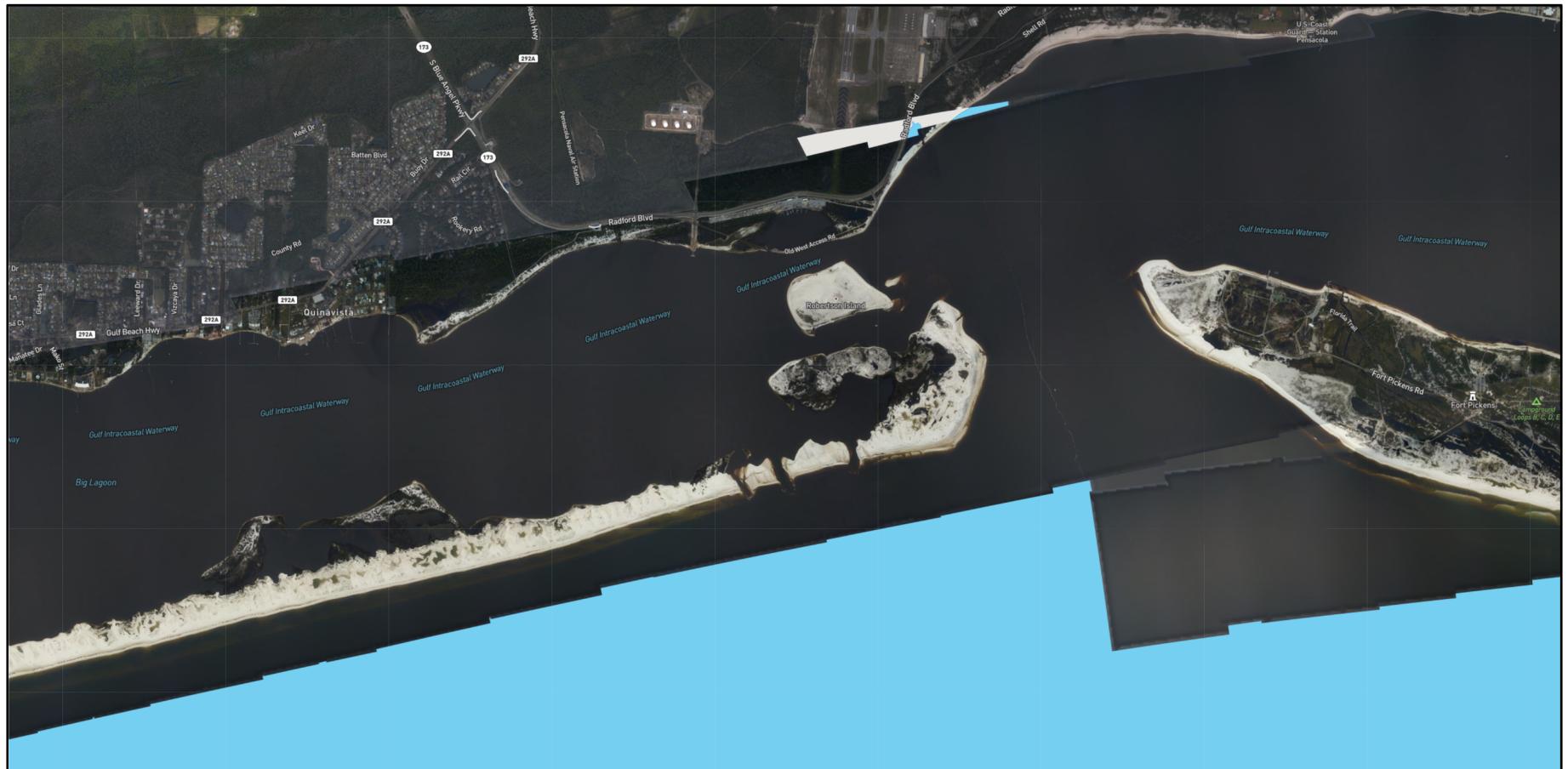
Figure 11. NOAA National Geodetic Survey aerial damage assessment image after Hurricane Sally showing three new cuts through Johnson Beach, Florida, on the eastern end of Perdido Key.
